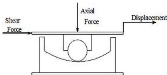
Fig. 8 Model of Friction Pendulum™ sliding bearing
