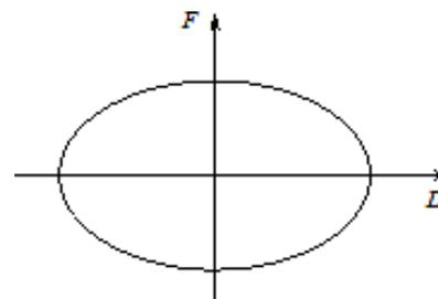
Fig. 9 Viscous fluid force-displacement loop
