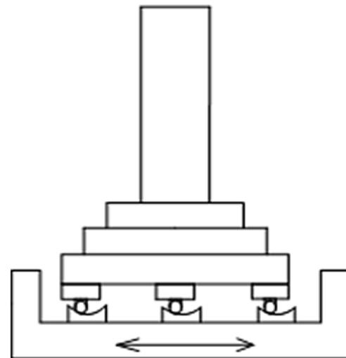
b) Seismic isolated structure
