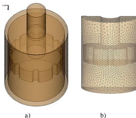
Fig. 11 a) The 3D model; b) the mesh of the fluid viscous damper (FVD)
