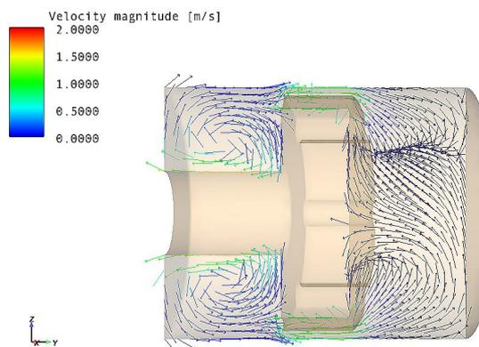
Fig. 13 Velocity magnitude of the fluid flow
