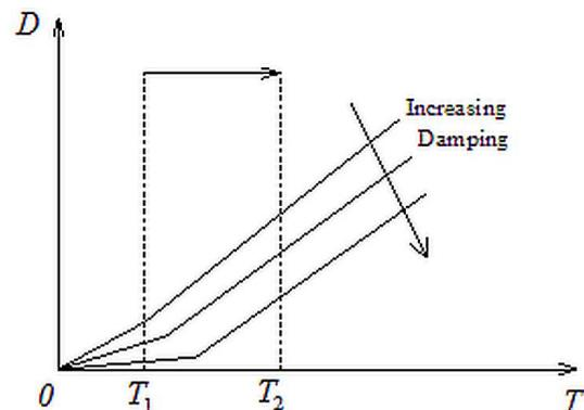
Fig. 6 The immediate effect of a seismic isolation system for three different damping levels
