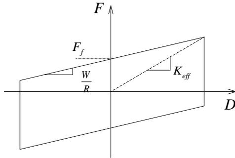
Fig. 7 Idealized sliding bearing hysteresis loop
