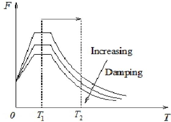
Fig. 5 Increasing the vibration period of the structure is reducing the base shear
