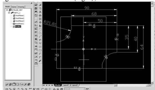
Fig. 3 Sizing and imposing constrains
