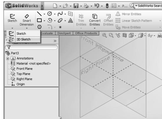
Fig. 12 Positioning of "3D Sketch"
