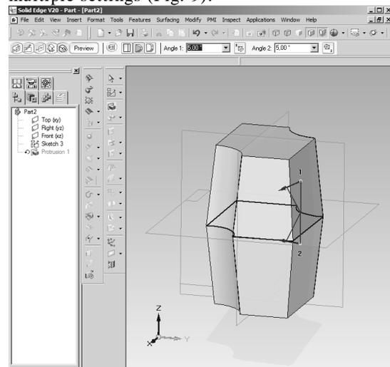
Fig. 8 "Draft" option of "Protrusion" command
