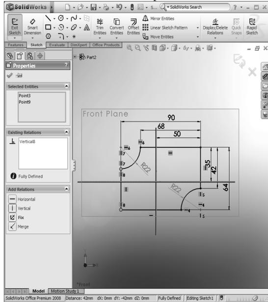
Fig. 13 Inserting constraints for points
