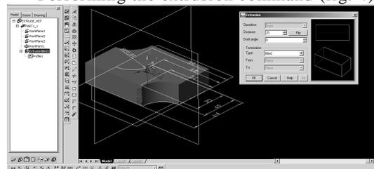
Fig. 4 Performing the extrusion command
