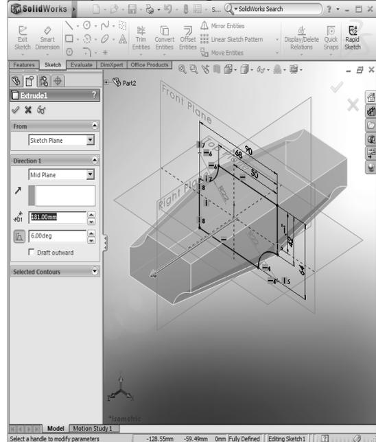
Fig. 16 "Draft" option of "Extrude" command
