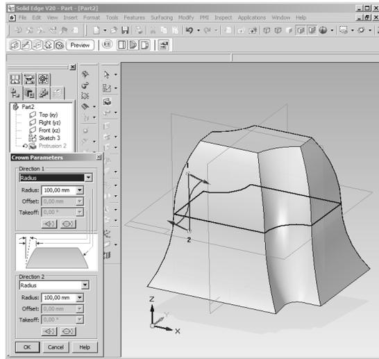
Fig. 9 Parameters of "Crown" option
