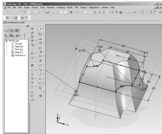
Fig. 10 Dynamic editing of "Protrusion"
