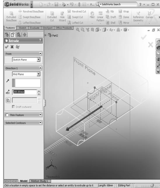
Fig. 15 Dynamic visualization of "Extrude" command
