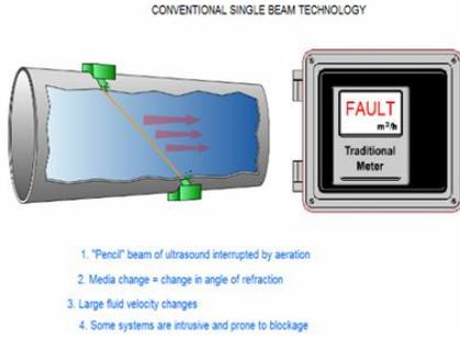
Fig. 5 Single beam technology flow measurement
