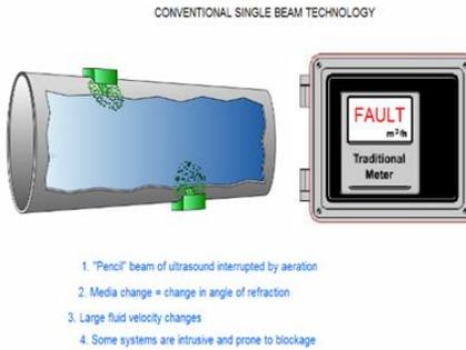
Fig. 6 Single beam technology flow measurement
