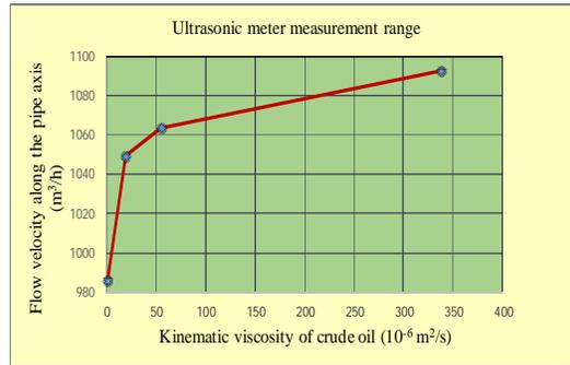
Fig. 13 Optimized Performance of Liquid Ultrasonic Meter Measurement Range
