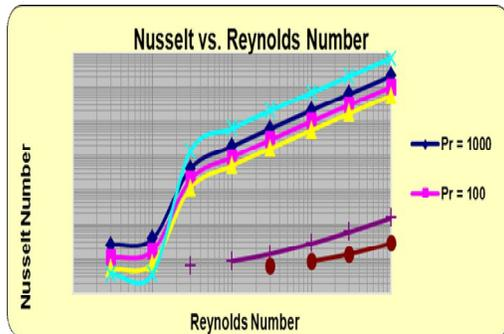
Fig. 11 Internal Flow Correlation for Heavy oil viscosity at 20°C
