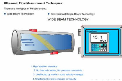
Fig. 3 Wide beam technology flow measurement
