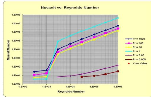
Fig. 12 Internal Flow Correlation for Extra heavy oil at 20°C
