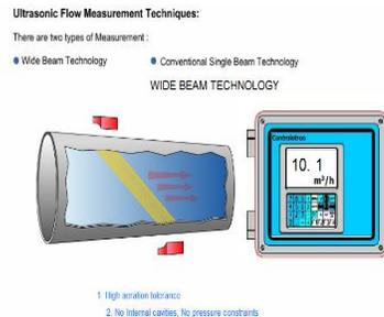
Fig. 4 Wide beam technology flow measurement
