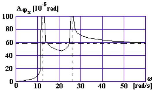
Fig. 5. The variation of the amplitude of the pitching rotation forced vibration phi\_x (inertial vibrating screen with 5m<sup>2</sup> sieves)
