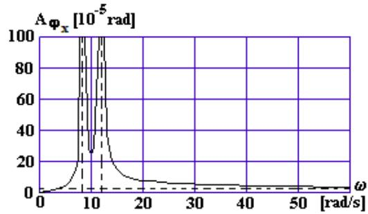
Fig. 7. The variation of the amplitude of the pitching rotation forced vibration phi\_x (inertial vibrating screen with 12m<sup>2</sup> sieves)
