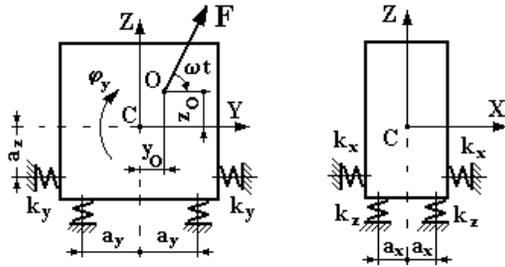
Fig. 3. Constructive scheme for the inertial vibrating screen with 12m<sup>2</sup> sieves
