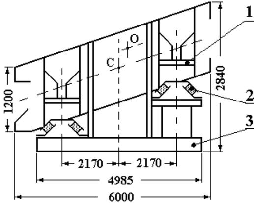
Fig. 2. Constructive scheme for the inertial vibrating screen with 12m<sup>2</sup> sieves
