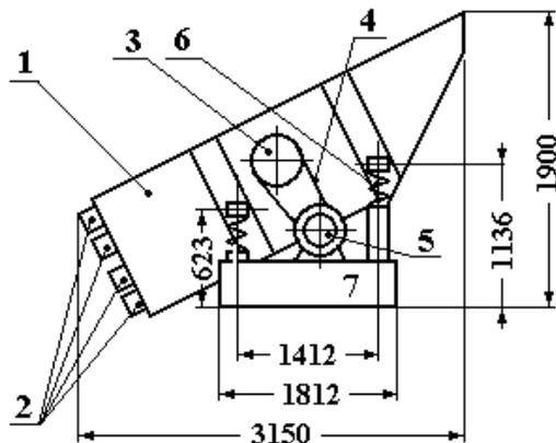
Fig. 1. Constructive scheme for the inertial vibrating screen with 5m<sup>2</sup> sieves
