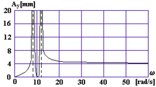
Fig. 6. The variation of the amplitude of the forced vibration on direction Y (inertial vibrating screen with 12m<sup>2</sup> sieves)
