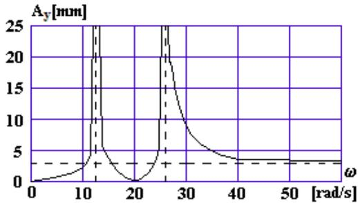
Fig. 4. The variation of the amplitude of the forced vibration on direction Y (inertial vibrating screen with 5m<sup>2</sup> sieves)
