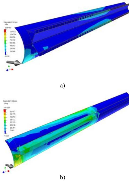
Fig. 5. Equivalent stress into the material of the two blades
