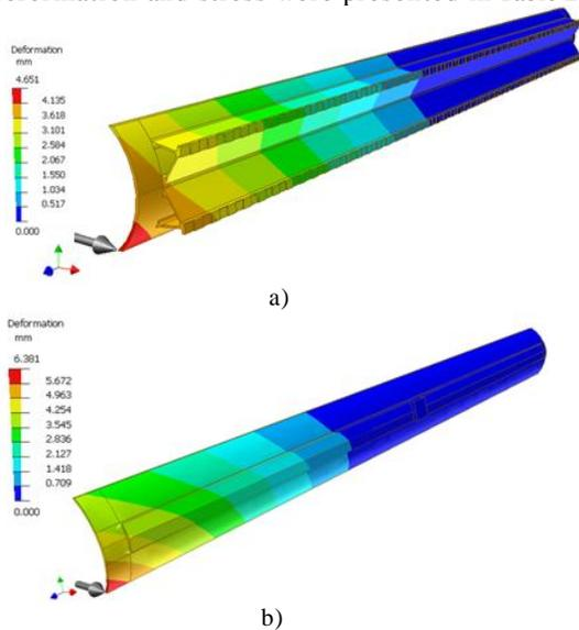
Fig. 4. Deformations of the two blades
