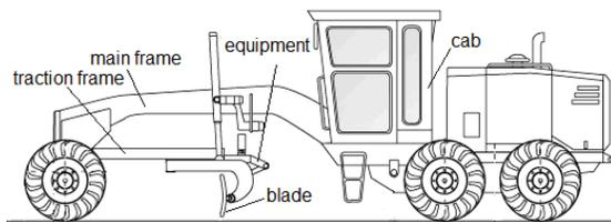
Fig. 1. The main grader's components
