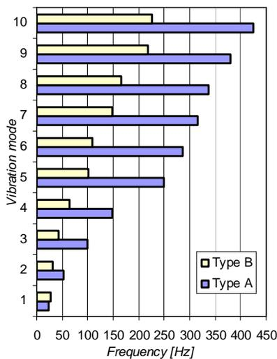
Fig.7. Comparative analysis of natural frequencies for the two types of blade
