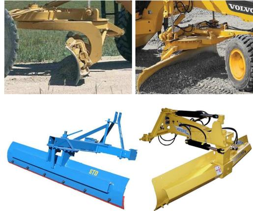
Fig. 2. Constructive solutions for the grader's blade (Caterpillar, Volvo, John Deere models)
