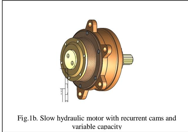
Fig.1b. Slow hydraulic motor with recurrent cams and variable capacity
