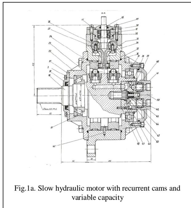
Fig.1a. Slow hydraulic motor with recurrent cams and variable capacity
