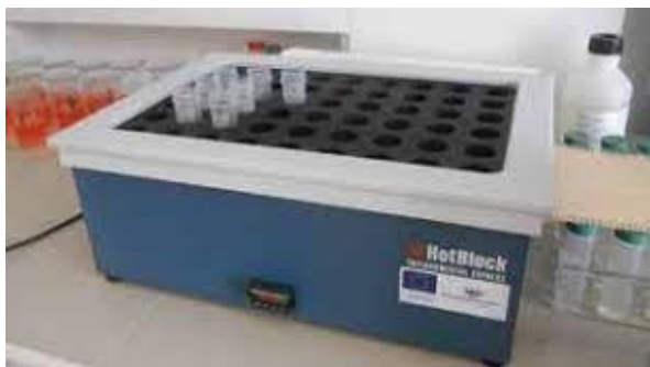
Fig. 2.2. Digester for liquid samples, HotBlock SC 151 (Environmental Express).
