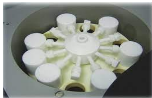
Fig. 2.3. Microwave digester for solid and semi-liquid samples, SpeedWave four SW-4 (Berghof)
