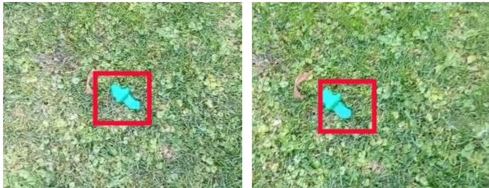
Fig. 2. Camouflaged 3D-printed PFM-1 in vegetated scene and corresponding DCDN segmentation result
