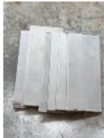
Fig. 3. Specimens in the form of rectangular plates before the hot forging process
