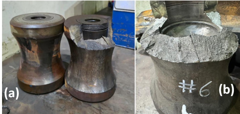
Fig. 1. Broken guide at site
