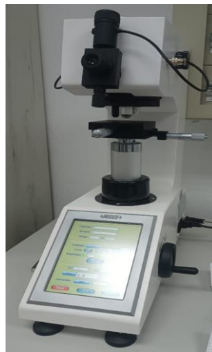
Fig. 1. Micro-Vickers HDT-VS1D INSIZE hardness tester
