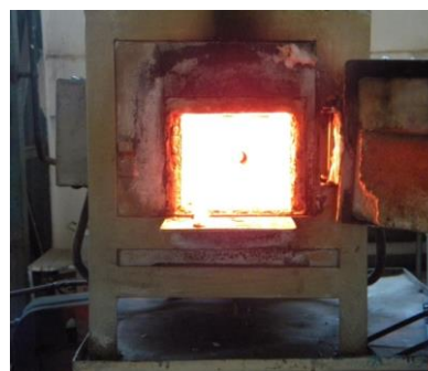
Fig. 1. Electric furnace used in experimental regimes of thermal processing on laboratory scale
