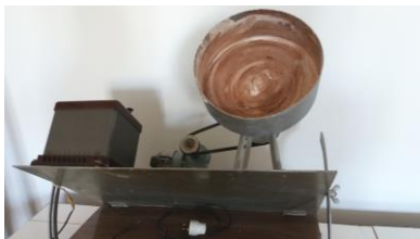
Fig. 4. Laboratory installation for pelletization
