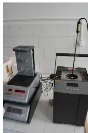
Fig. 7. Calibration thermobalance sensor at 15°, 20° and 30 °C
