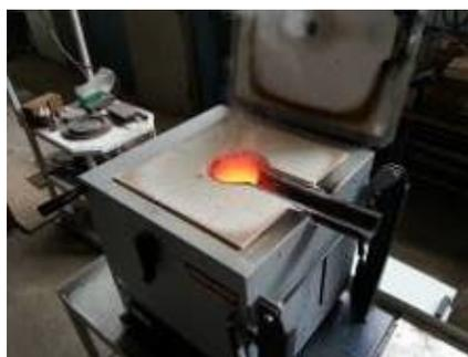
**Fig. 2.** Electric crucible furnace for copper wire scrap melting
