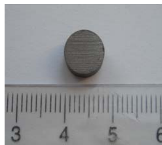
Fig. 3. Worn surface after the abrasion test
