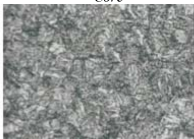
Center hardness: 329 HV
