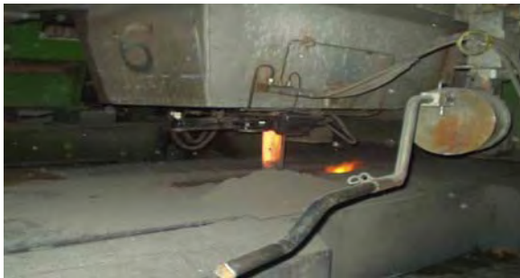
Fig. 7. Tube changer in operation on the slab caster no.1 in Mittal Steel Galati [3]
