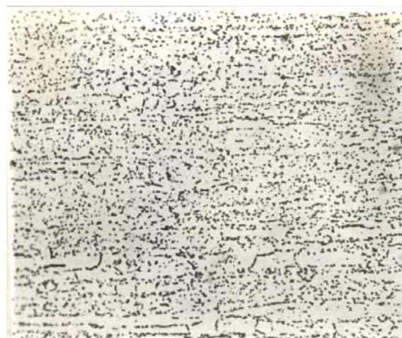
Fig.5. Microstructure 231667 coil no. (laboratory thermal treated): a. annealing 2 hours at 810 o C, b. annealing 12 hours at 810 o C. Attack: oxalic acid 10%, magnify: 500:1.
