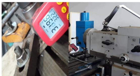
Fig. 2. Shows device those measurers the temperature by distance
