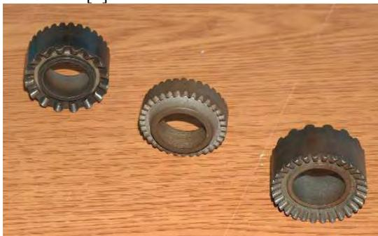
**Fig. 5.** Sintered satellites from P/M for precessional transmissions.
