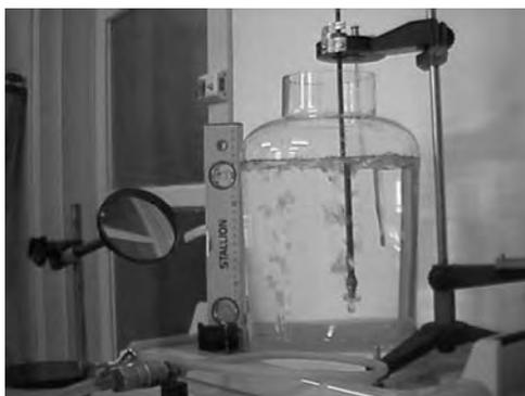
**Fig. 13** Water model vessel.
