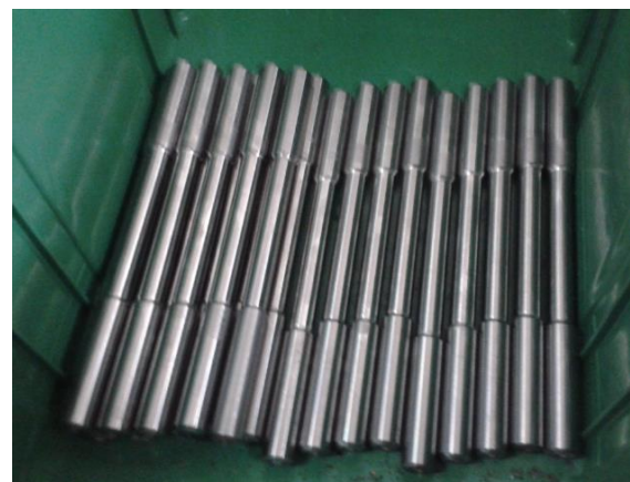
Fig. 19. Samples test for hot tensile test
