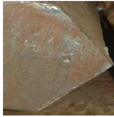
Fig. 13. Chamfering at both ends of the cut addition
