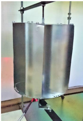
Fig. 10. Experimental model with 4 semi-cylindrical cups (S4CNL) fixed on the test frame
