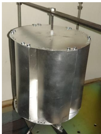
Fig. 12. Experimental model with 6 semi-cylindrical cups (S6CNL) fixed on the test frame
