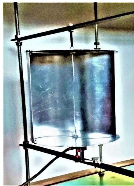
Fig. 8. Experimental model with 2 semi-cylindrical cups (S2CNL) fixed on the test frame
