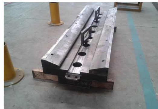
Fig. 4. Lower die of bending press with opening of 500 mm
