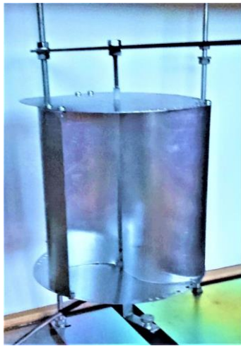
Fig. 9. Experimental model with 3 semi-cylindrical cups (S3CNL) fixed on the test frame
