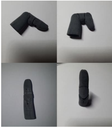
Fig. 4. 3D printing results of the custom index finger prosthesis
