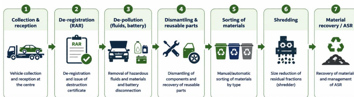
Fig. 6. Technological Workflow of an Authorized End-of-Life Vehicle (ELV) Treatment Facility
