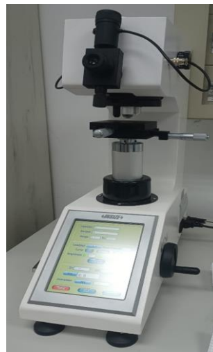
Fig. 1. Micro-Vickers HDT-VS1D INSIZE hardness tester
