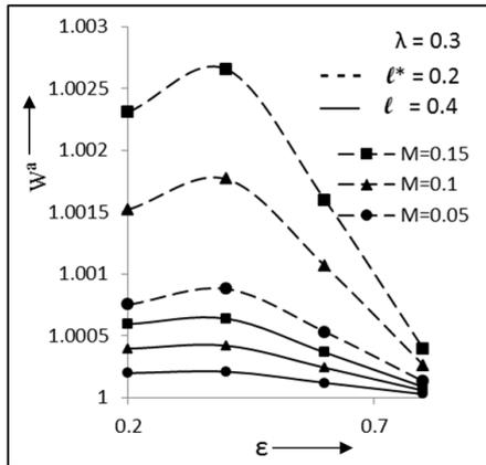
Fig. 4.5. Variation of Normalized load capacity as variation of eccentricity ratio for rotation parameter
