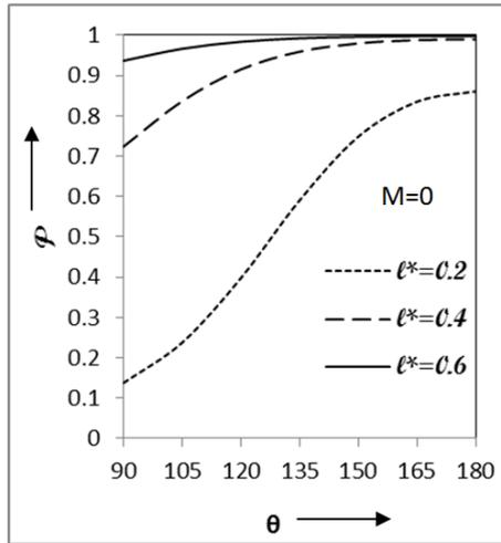
Fig. 4.1. Variation of Normalized pressure as variation of  $\theta$  for couple stress parameter at no rotation
