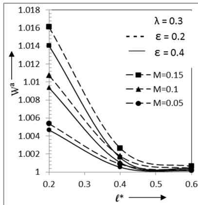
Fig. 4.6. Variation of Normalized load capacity as variation of couple stress parameter for rotation parameter
