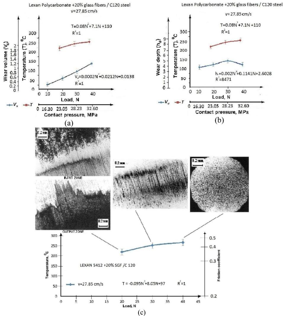
**Fig. 11.** The evolution in contact temperatures and wear appearance at speeds of 27.85 cm/s, for PC Lexan 3412 + 20% SGF / C120
