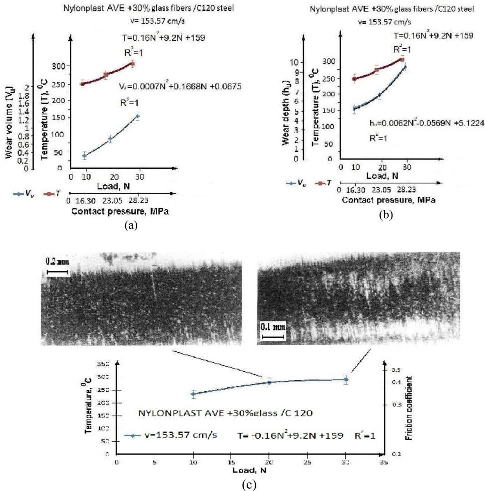
Fig. 8. Wear evolution of the scar wear volume (a) and depth (b) as a function of the normal load and contact temperature and the variation in contact temperature (c) as a function of the normal load and friction coefficient at the sliding speed of 153.57 cm/s, for Nylonplast AVE Polyamide + 30% SGF / C120 steel grade
