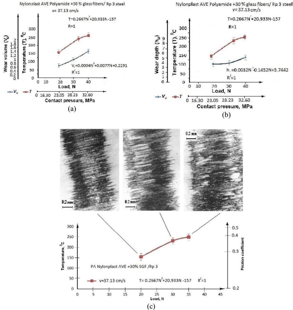
**Fig. 9.** Wear evolution of the scar wear volume (a) and depth (b) as a function of the normal load and contact temperature and the variation in contact temperature (c) as a function of the normal load and friction coefficient at the sliding speed of 37.13 cm/s, for Nylonplast AVE Polyamide + 30% SGF / Rp3 steel grade
