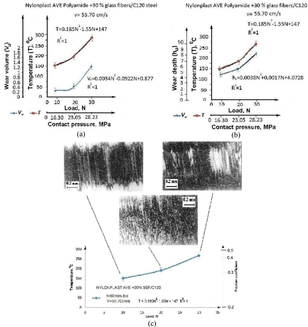
**Fig. 6.** Wear evolution of the scar wear volume (a) and depth (b) as a function of the normal load and the contact temperature and the variation in contact temperatures (c) as a function of the normal load and friction coefficient at the sliding speed of 55.70 cm/s, for Nylonplast AVE Polyamide + 30% SGF / C120 steel grade
