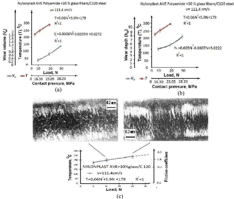
**Fig. 7.** Wear evolution of the scar wear volume (a) and depth (b) as a function of the normal load and contact temperature and the variation in contact temperature (c) as a function of the normal load and friction coefficient at the sliding speed of 111.4 cm/s, for Nylonplast AVE Polyamide + 30% SGF / C120 steel
