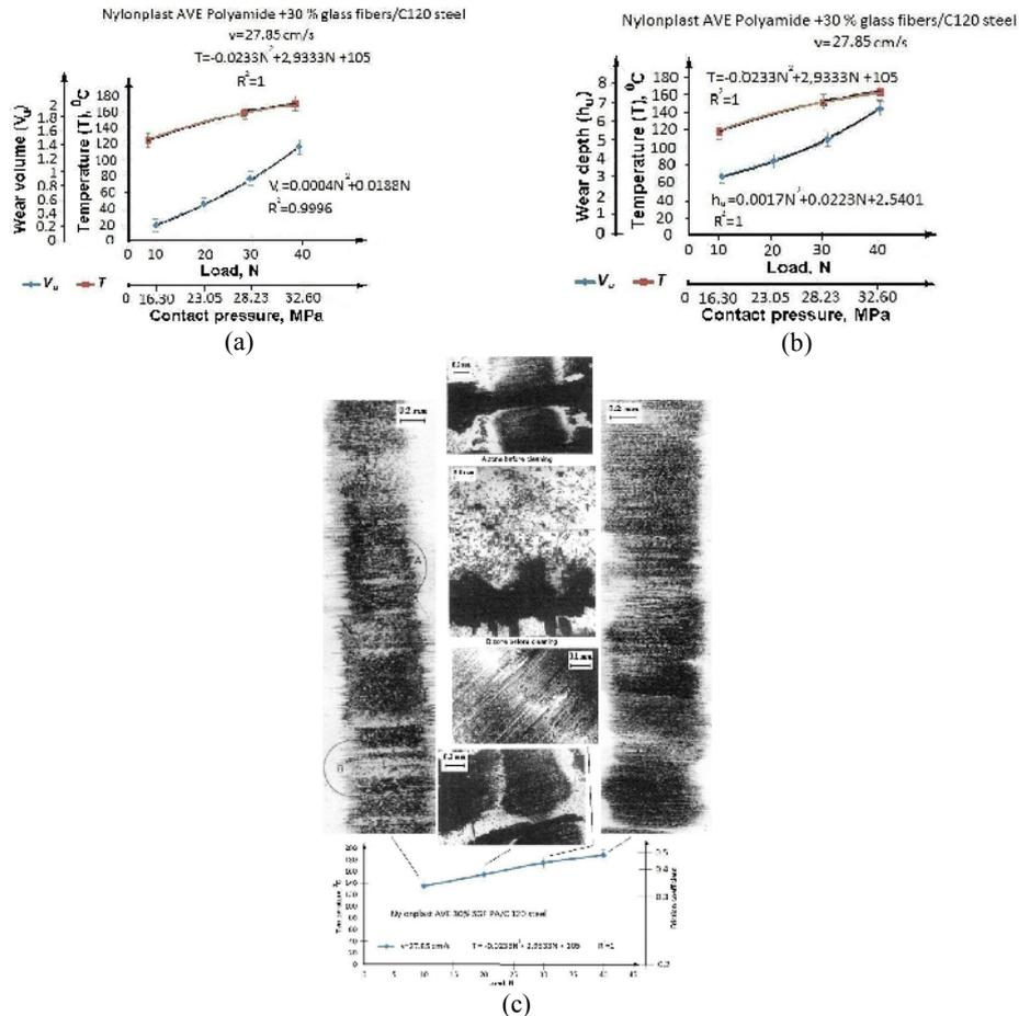
**Fig. 4.** Wear evolution of the scar wear volume (a) and depth (b) as a function of the normal load and the contact temperature and the variation in contact temperature (c) as a function of the normal load and the friction coefficient at the sliding speed of 27.85 cm/s, for Nylonplast AVE Polyamide + 30% SGF / C120 steel grade
