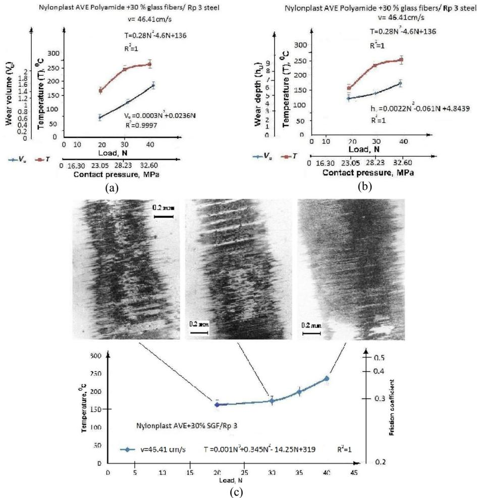
**Fig. 10.** Wear evolution of the scar wear volume (a) and depth (b), as a function of the normal load and contact temperature and the variation in contact temperature (c) as a function of the normal load and friction coefficient at the sliding speed of 46.41 cm/s, for Nylonplast AVE Polyamide + 30% SGF / Rp3 steel grade
