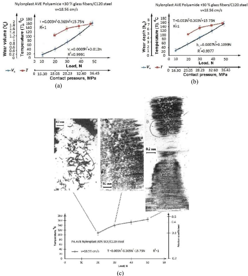
**Fig. 2.** Another aspects of wear evolution as scar wear volume (a) and depth (b) function of the normal load and the contact temperature and variation of wear mode (c) depending of the contact temperature and the normal load, at speed sliding of 18.56 cm/s, for Nylonplast AVE Polyamide + 30% SGF / C120 steel
