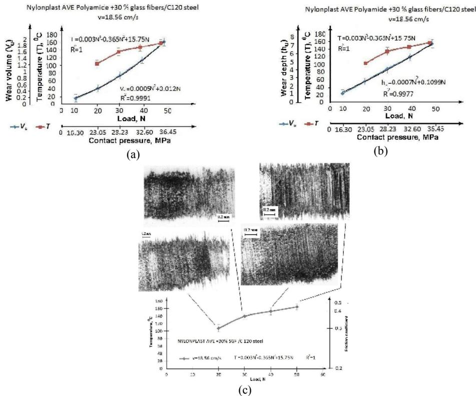
Fig. 1. Wear evolution as a scar wear volume (a) and depth (b) function of the normal load and the contact temperature and the variation of the contact temperature (c) as a function of the normal load and friction coefficient at the sliding speed of 18.56 cm/s, for Nylonplast AVE Polyamide + 30% SGF / C120 steel
