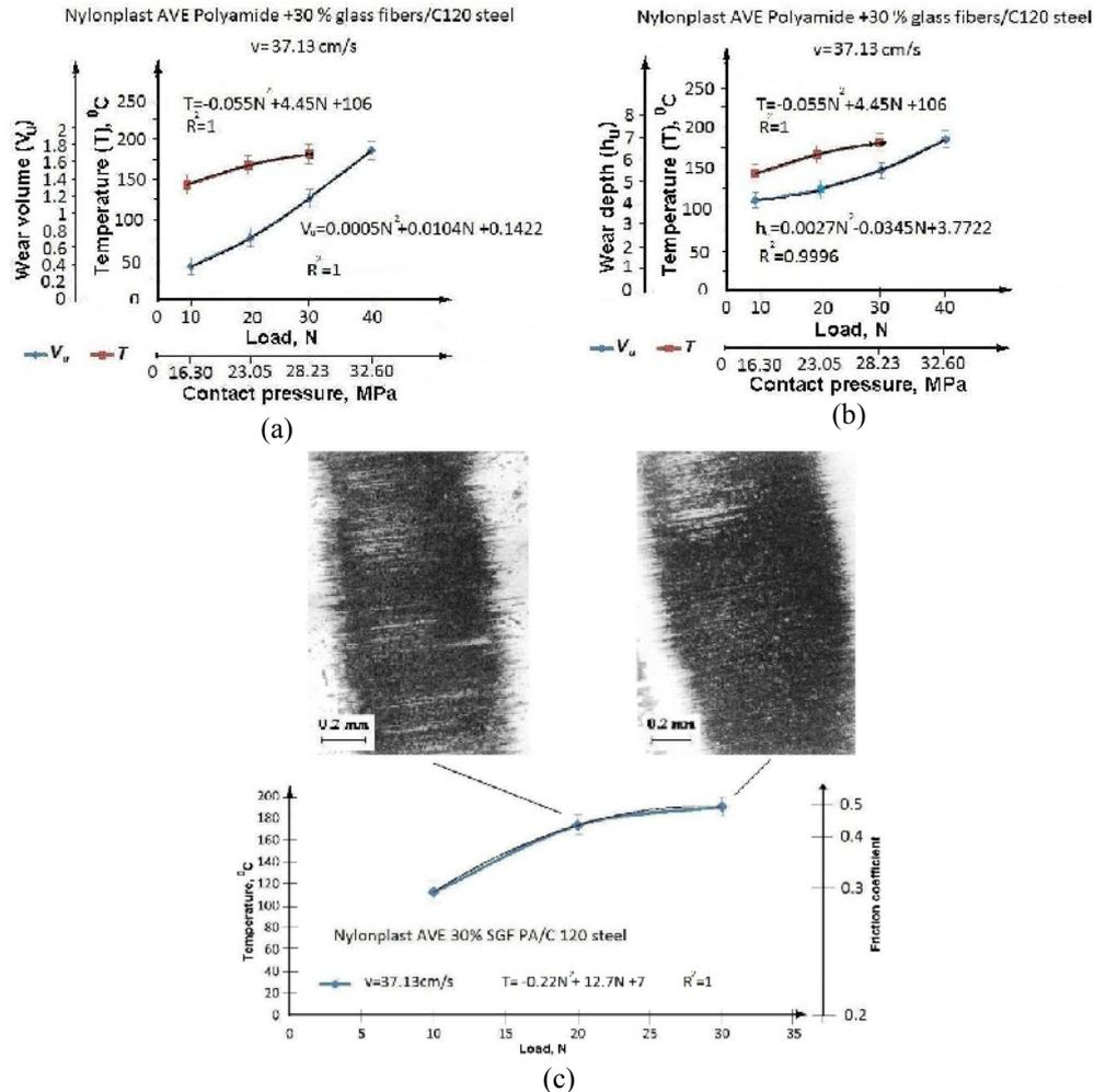
**Fig. 5.** Wear evolution of the scar wear volume (a) and depth (b) as a function of the normal load and the contact temperature and the variation in contact temperature (c) as a function of the normal load and the friction coefficient at the sliding speed of 37.13 cm/s, for Nylonplast AVE Polyamide + 30% SGF / C120 steel grade
