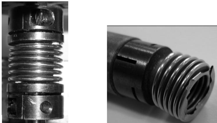
Fig. 4. Actual corrugated bellow and the broken one
