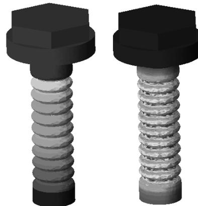
**Fig. 7.** The deformations and von Mises stresses for the first vibration mode
