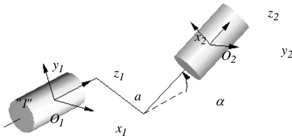
**Fig. 2.** The parameters and the reference systems used for characterizing the relative position of the two shafts
