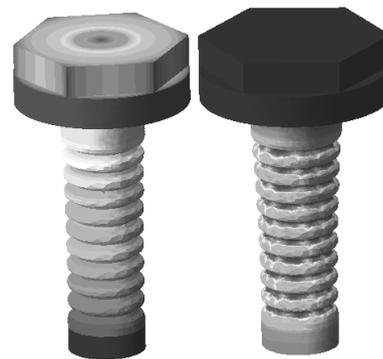
**Fig. 8.** Deformations and von Mises stresses for the second vibration mode,  $f = 730.51\text{Hz}$
