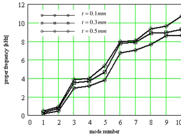
**Fig. 10.** The natural vibration frequencies corresponding to the first ten vibration modes for three metal sheet thickness,  $t$
