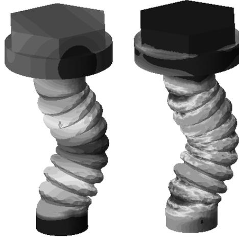
**Fig. 9.** The deformations and von Mises stresses for the third vibration mode,  $f = 3540.86Hz$
