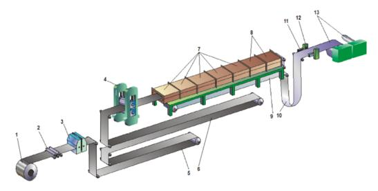
Fig. 2. *Dip pickling line*
