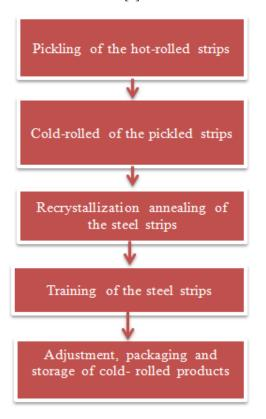
Fig. 1. Cold rolled steel manufacturing process
