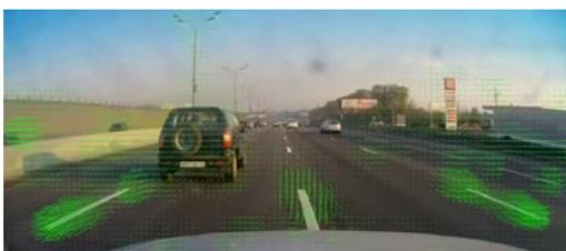
**Fig. 1.** Vector motion as identified by the flow motion detector
