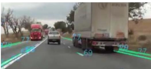
**Fig. 7.** Detection of lane markings
