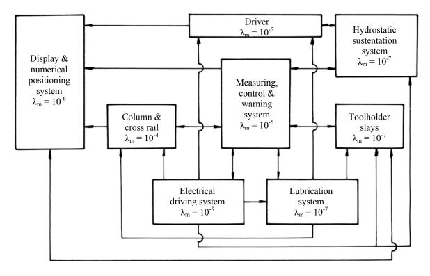
Fig. 3. Interconnections in assessing a vertical lathe reliability
