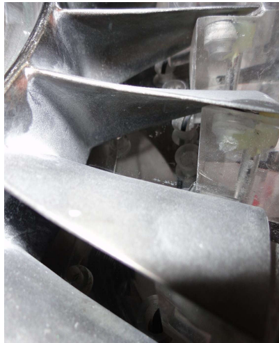
Fig. 1. Speakers positioned to lie parallel to the blade faces
