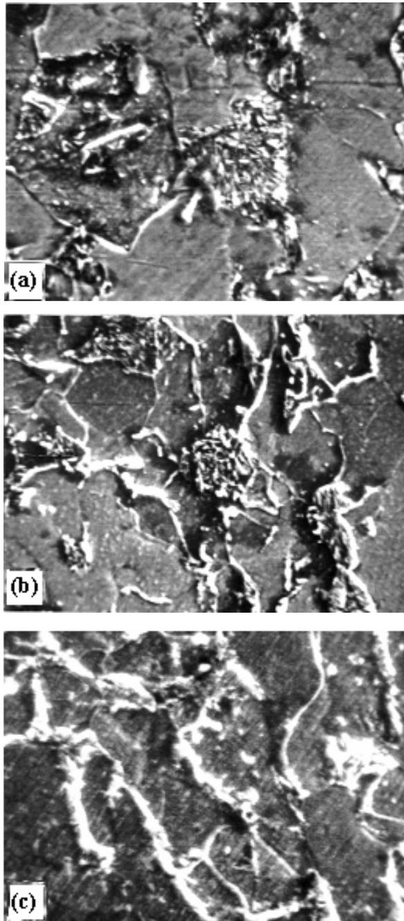
Figure 6. SEM micrographs of AISI 1015 steel after different soaking times at 650°C: a - 30 min.; b - 1 h; c - 2 h; d - 3 h (magnification 5000:1).
