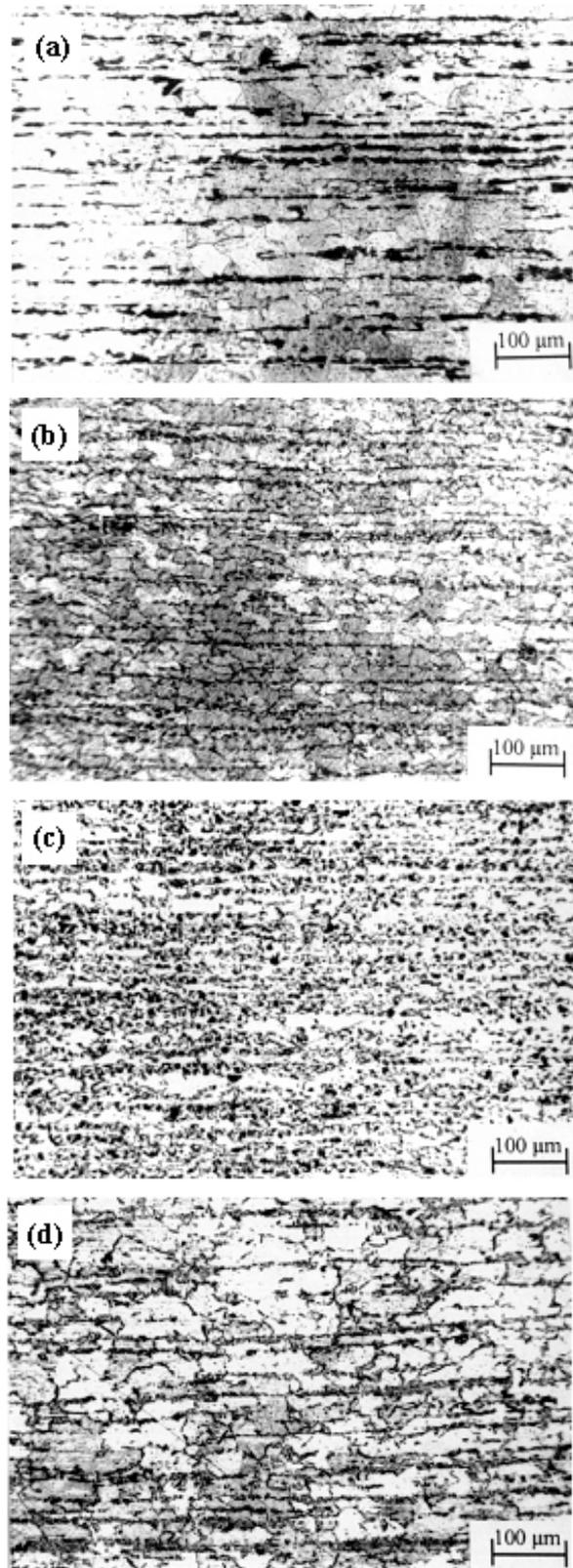
Figure 5. Microstructure of steel AISI 1015 after different soaking times at 650 °C: a - 5 min.; b - 30 min.; c - 3 h; d - 8 h. ( optical microscopy)
