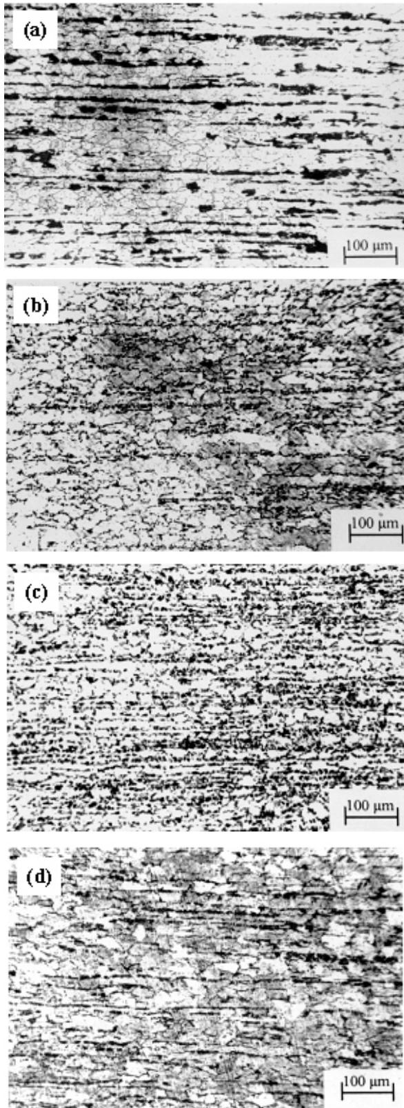
Figure 4. Microstructure of 0.15 % C steel after different soaking times at 600 °C: a - 10 min.; b - 30 min.; c - 3 h; d - 8 h.
