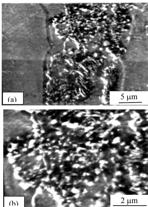
Figure 2. Microstructural modifications of the pearlite after warm rolling assessed by electron microscopy (SEM). Magnification (a) 5000:1, (b) 10000:1.
