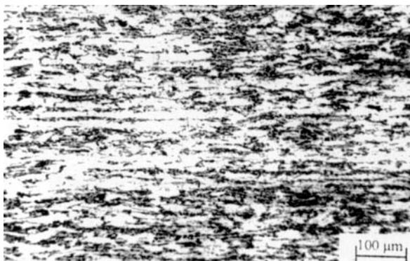
Figure 1. Microstructure of steel AISI 1015 after warm rolling.
