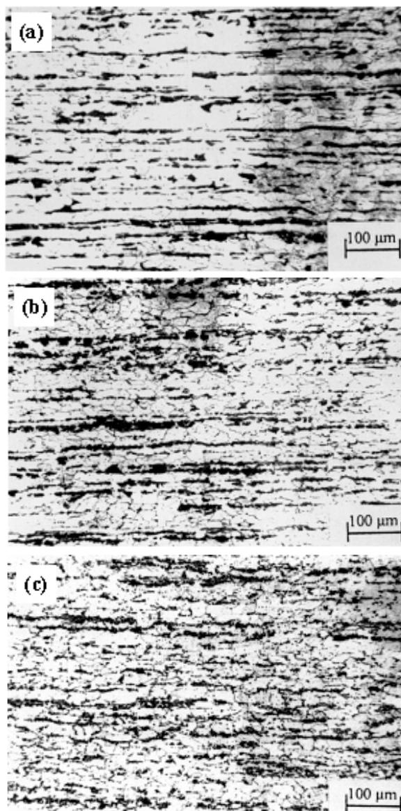
Figure 3. Microstructure of AISI 1015 steel after different soaking after different soaking times at 550 °C: a - 10 min.; b - 2 h; c - 10 h
