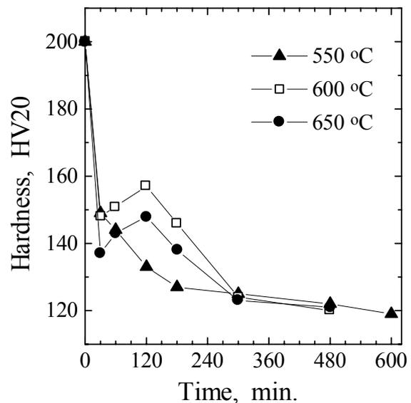
Figure 6. The influence of the temperature and the soaking time on the hardness of 0.15% C steel.
