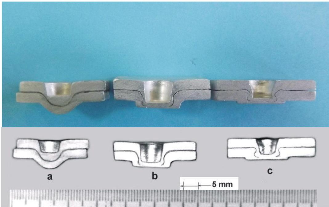
Fig. 8. Macroscopic aspect of specimens after execution stages: a – free embossing; b – welding + riveting; c – flattening
