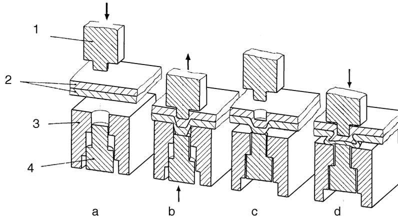
**Fig. 6.** Mechanical joining by riveting without local perforation:
