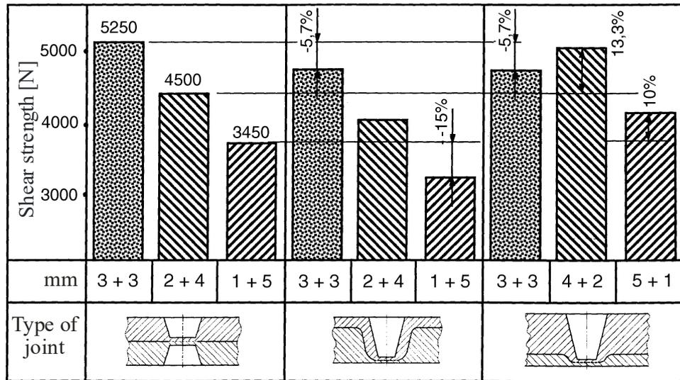
Fig. 4. Shear strength for different assemblies of Al 99.5 sheets using punches with diameter  $d = 8$  mm
