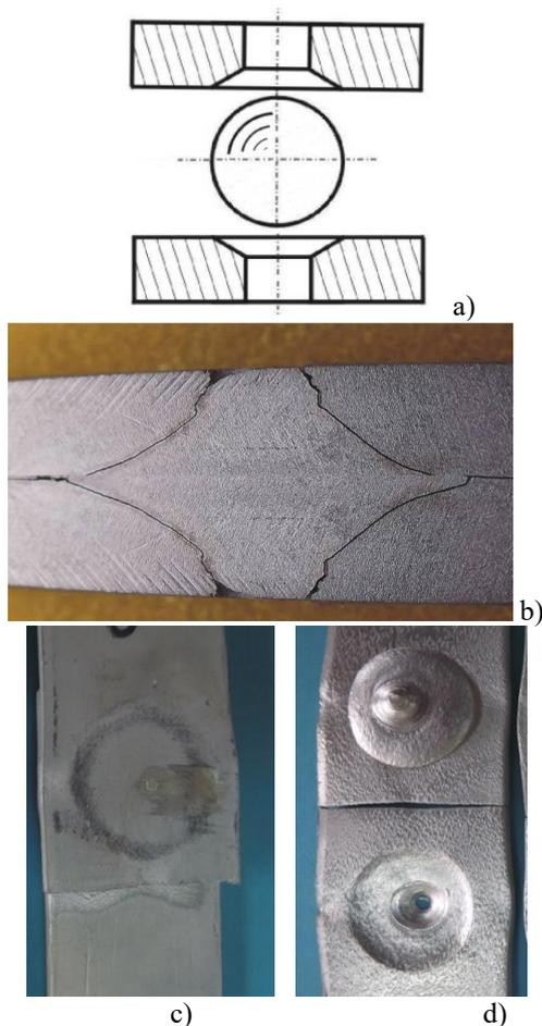
**Fig. 13.** Assembly with perforated and countersunk plates
