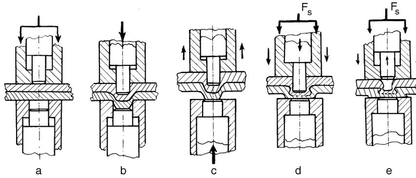
Fig. 7. Cold spot welding combined with self-piercing joining, using coaxial punches
