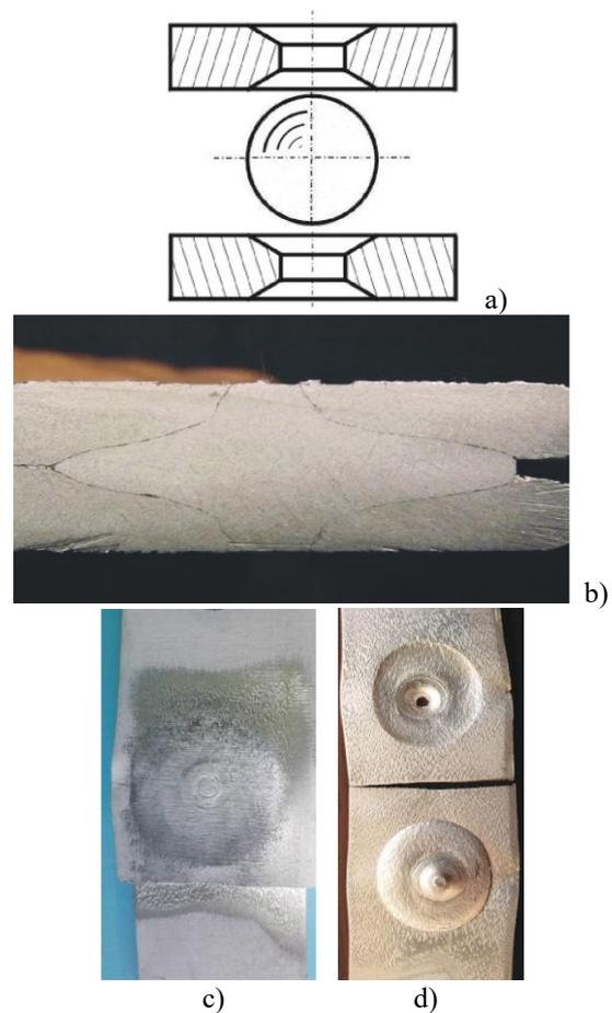
**Fig. 14.** Welding with drilled and double-countersunk plates
