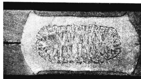
**Fig. 1.** Macrostructure of a welded spot
