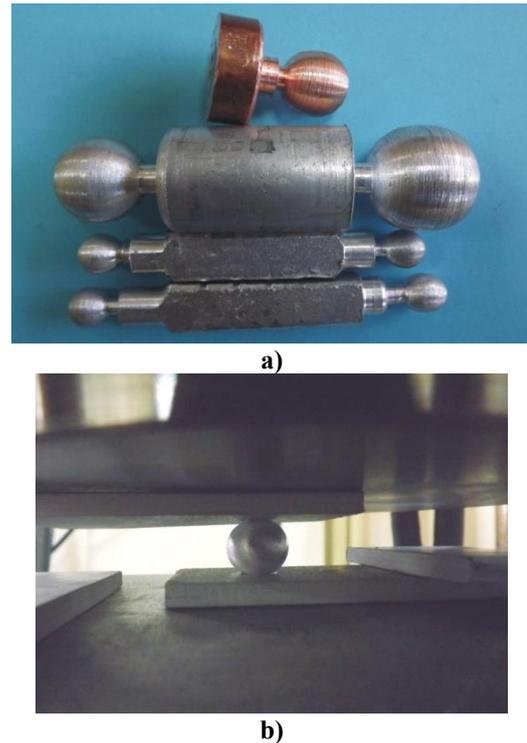
**Fig. 10.** Preparation of the spherical intermediate element and pressing with flat plates
