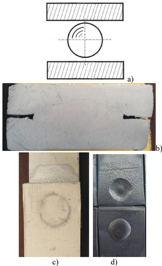
**Fig. 11.** Cold welding with flat plates and a spherical intermediate element
