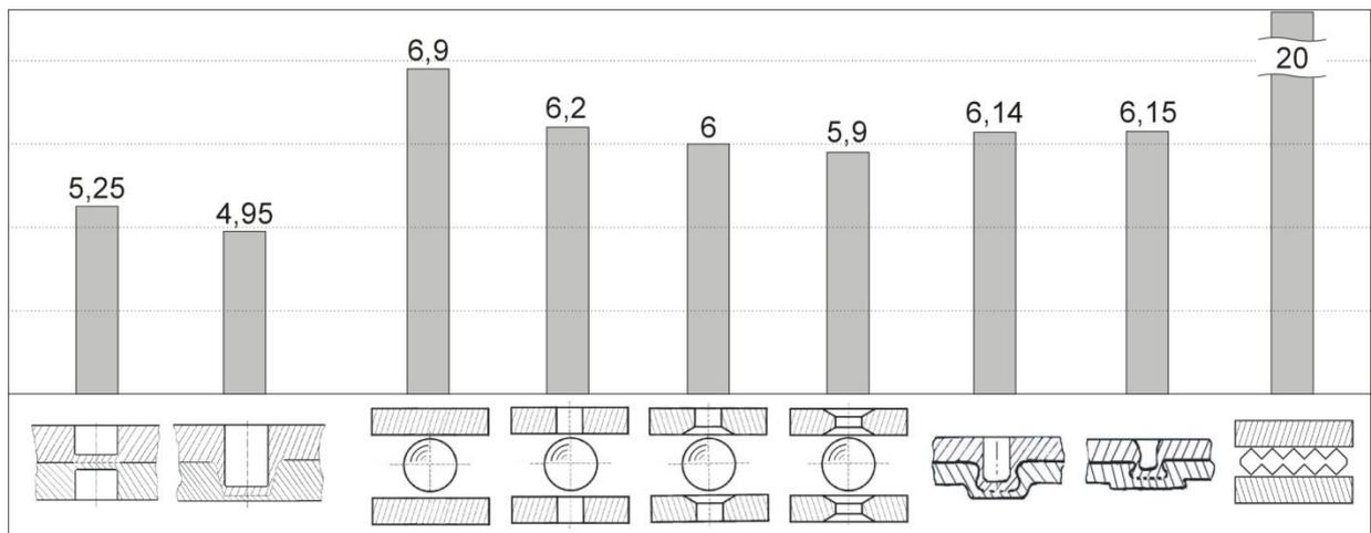
Fig. 15. Shear strength of various cold pressure spot welds [kN]
