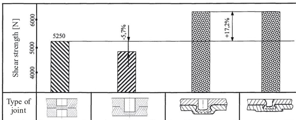
Fig. 9. Shear strength of cold spot welded joints vs. welded + riveted joints, with or without additional flattening
