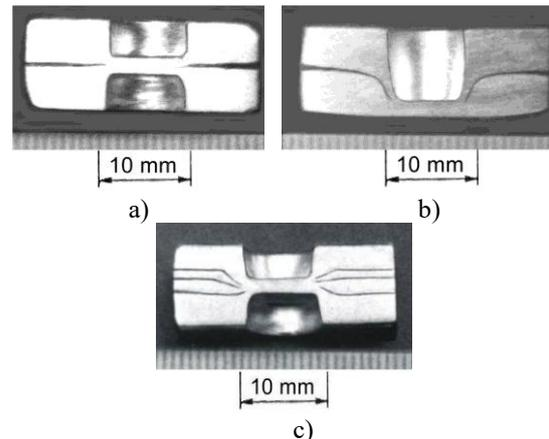
Fig. 3. Macroscopic aspect of aluminium specimens welded by cold pressure welding
