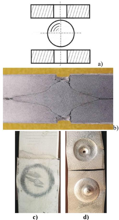
**Fig. 12.** Cold welding with perforated plates and a spherical intermediate element
